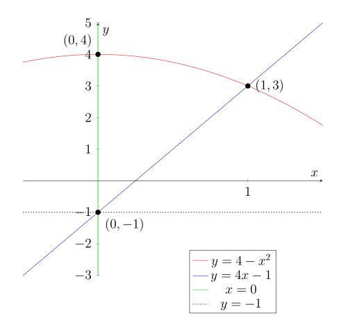
After rotating the region about y = -1, a typical cross-section cut parallel to the y-axis (say, at  $x = x_0$ ) looks like this:
